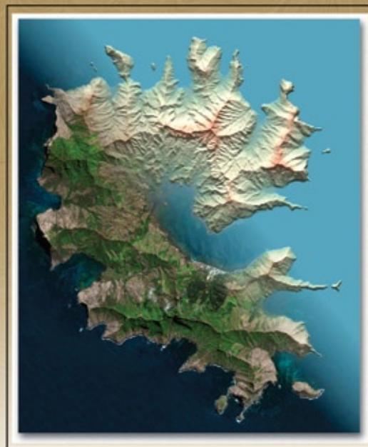
A digital elevation model (DEM) of Rapa, French Polynesia, photogrammetrically derived from IKONOS stereo satellite imagery. The digital terrain model was used to orthorectify QuickBird imagery (shown partially draped on top of the DEM).
